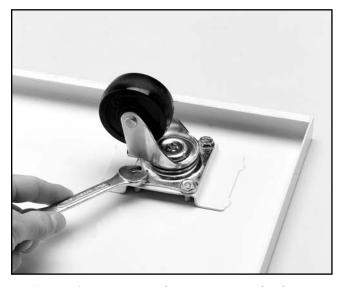
Figure 8. Mounting the casters to the base.
